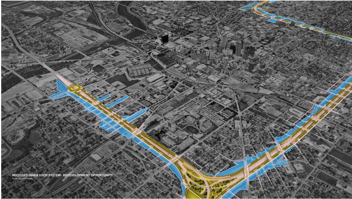
This image shows a recessed Inner Loop system with a compressed footprint freeing up State-owned interstate right-of-way (highlighted in blue) for redevelopment.
