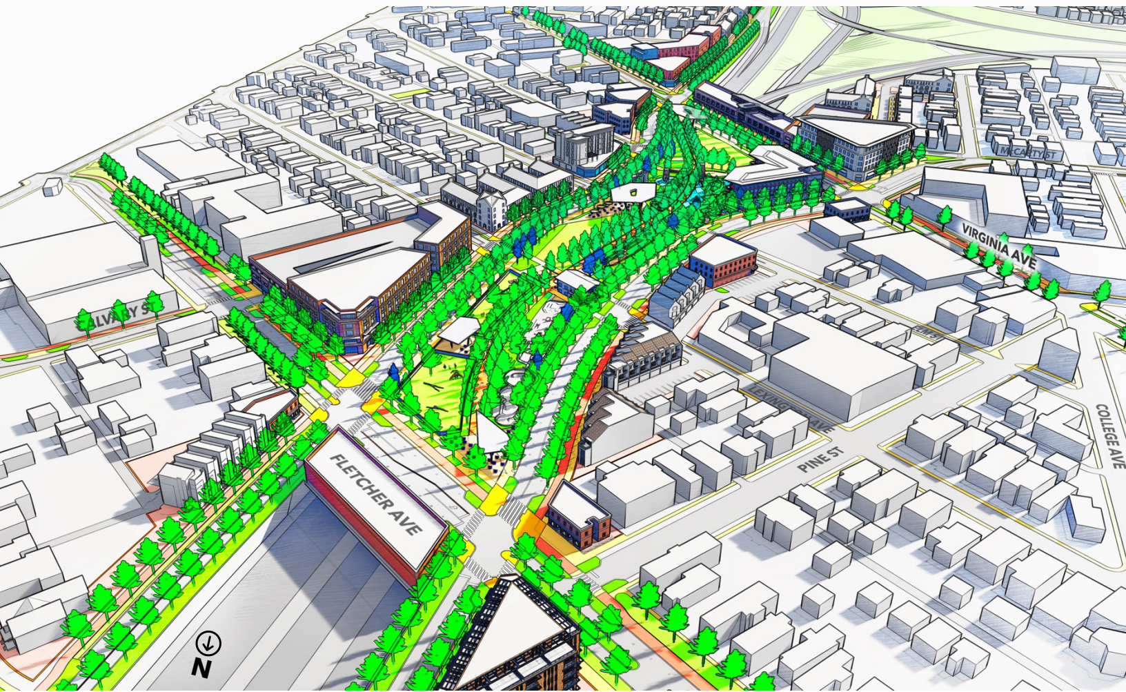
Illustration of cap constructed over the interstate reconnecting communities and creating new land for development.
