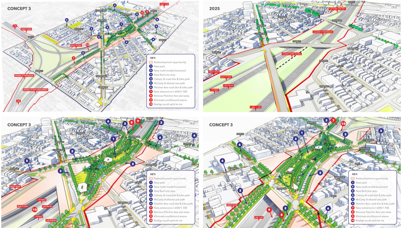
Images showing Concept 3 and its integration with the interstate right-of-way (red line) and newly developable land (highlighted in peach) previously in the interstate right-of-way.
